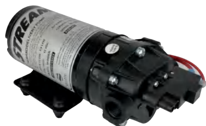
STREAMFLO® Pump 12v 100psi 5.5lpm 3/8F Threaded Ports
